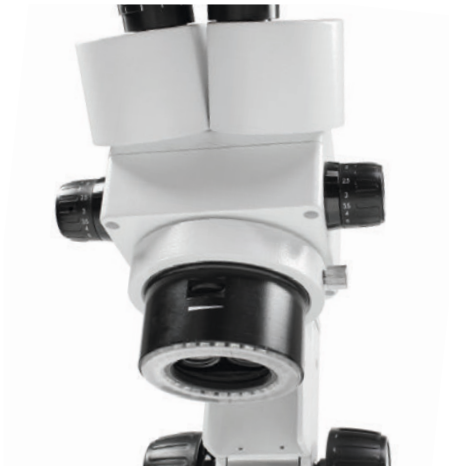
Dimmable, integrated LED ring illumination
