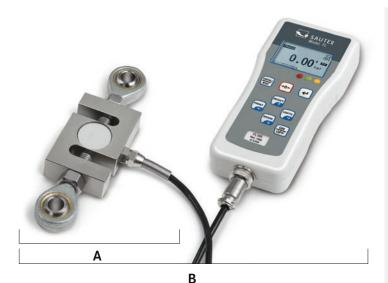
Situation A: Separate force transducer, display unit mV/V Situation B: Complete force gauge (N), consisting of transducer, amplifier and display, display unit N
