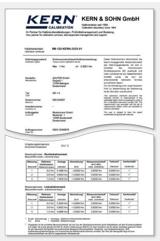
Factory calibration certificate for torque wrench test devices (extract from the factory calibration certificate) Further details on the internet at www.kern-lab.com
