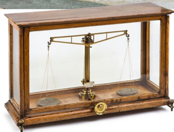
Precision balance around the year 1840, in glass housing with milligramme sensitivity
